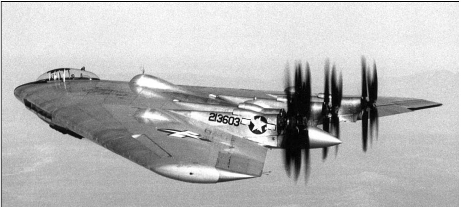
32 Northrop's Flying Wing Bomber known as the XB-35 in flight in 1946. The XB-35 was an experimental heavy bomber developed for the U.S. Army Air Force during World War II. The project was terminated shortly after the war, due to its technical difficulties. (AP Photo) # 📷
