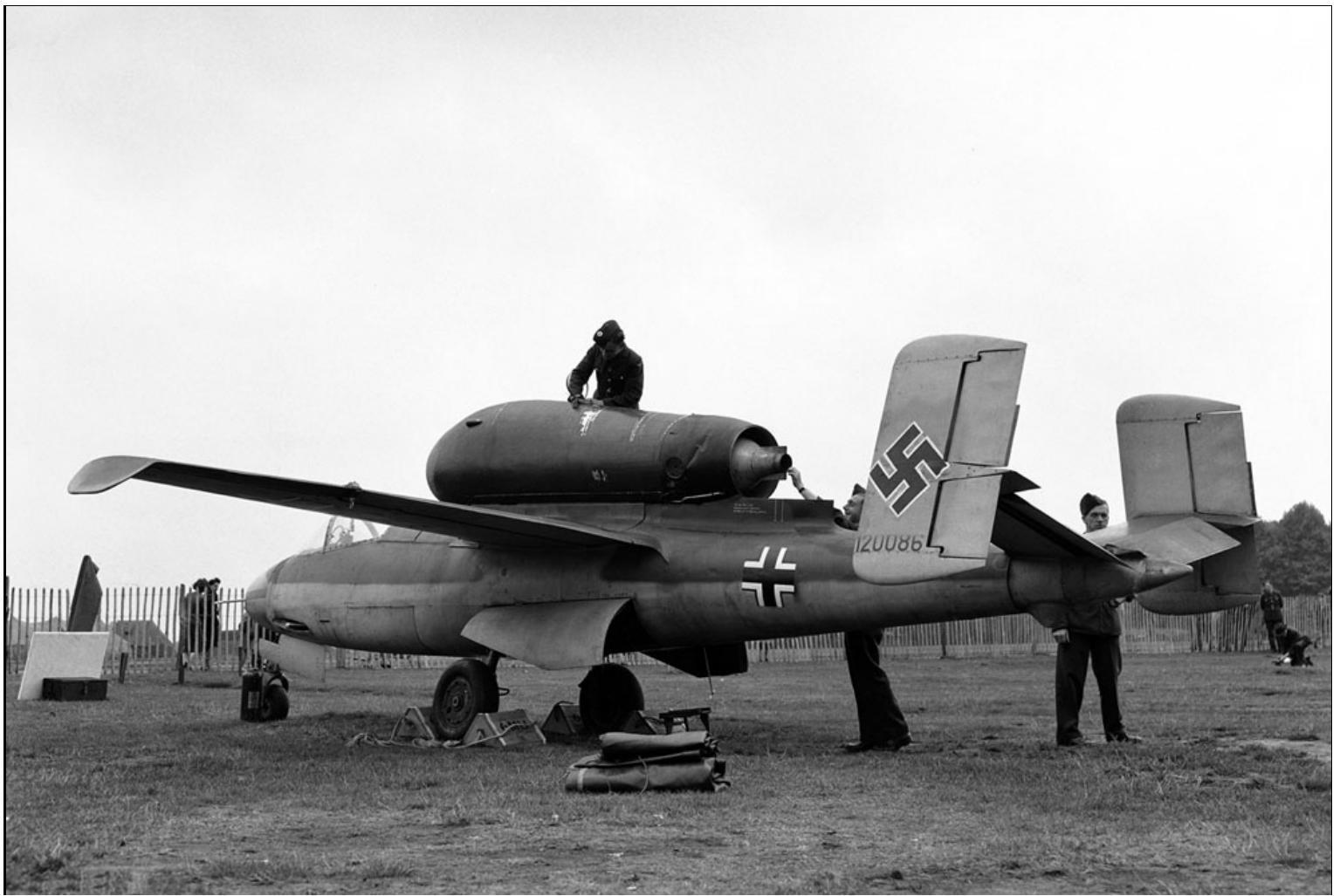
11 Many of Germany's captured new and experimental aircraft were displayed in an exhibition as part of London's Thanksgiving week on September 14, 1945. Among the aircraft are a number of jet and rocket propelled planes. Here, a side view of the Heinkel He-162 "Volksjaeger", propelled by a turbo-jet unit mounted above the fuselage, in Hyde park, in London. (AP Photo) # 🇩🇪
